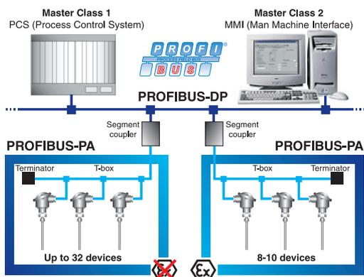
PROFIBUS is a fieldbus network for digital communication over a 2-wire architecture based on the international standard EN 50170. Two levels are used in a PROFIBUS network: the high level PROFIBUS-DP used for process control and the field level PROFIBUS-PA used for field instrumentation.
