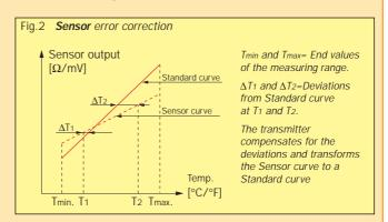
**System error correction** -This method is used to correct the system error (sensor + transmitter error) by exposing the sensor to one (one-point correction) or two (two-point correction) accurately measured temperatures (true temperatures). The true temperature(s) are entered, and the transmitter automatically corrects for the system errors. *Fig. 3*.
