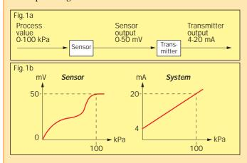
Exemple of a system (sensor + transmitter) with an output **linear** to the process value, in spite of a **non-linear** sensor.
