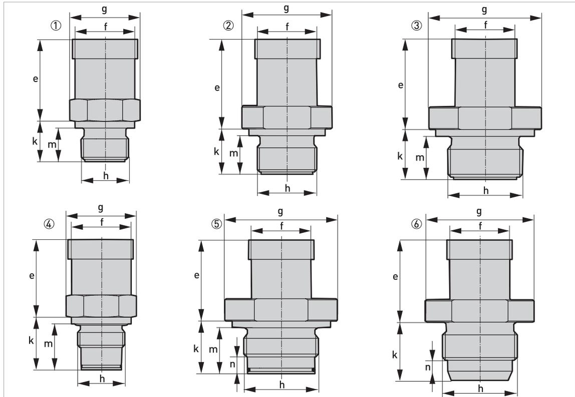
Figure 6-2: Dimensions for pressure transmitter with threaded connection
